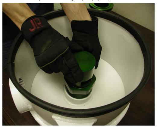
4. Place the bonnet, as shown below, on the plunger. We recommend lubricating mating surfaces with 30-weight oil. There should be a light film of oil on the plunger at all times.
