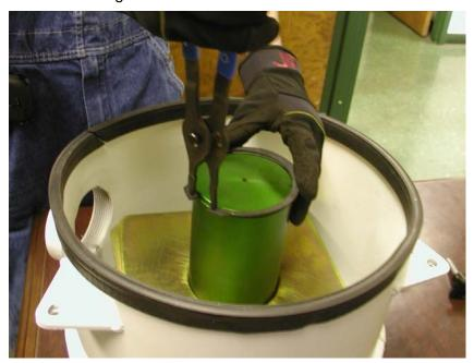
7. Line up the tabs with the lid. Secure the handles.
